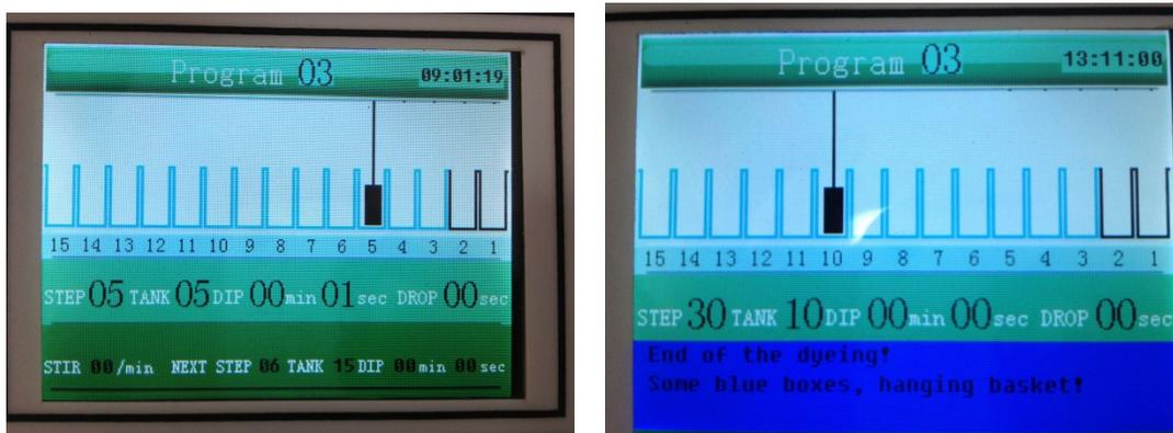
8) When the instrument finishes one program, the slide basket will stop either in the tank used in the last step or above the station 2 based on the selection in the step 5) and the machine will sound a buzzing alarm every 5 seconds to indicate that the program is finished. Please remove slide basket and touch the blue window (as shown above) to continue staining or turn off the instrument if finished. Or, press 'run' key to process another program.
