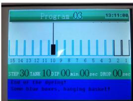
8) When the instrument finishes one program, the slide basket will stop either in the tank used in the last step or above the station 2 based on the selection in the step 5) and the machine will sound a buzzing alarm every 5 seconds to indicate that the program is finished. Please remove slide basket and touch the blue window (as shown above) to continue staining or turn off the instrument if finished. Or, press 'run' key to process another program.
