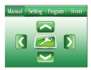
**2)** Select desired function. Then, press the middle key to enter into the password setting interface. Enter a figure from 1 to 9 in the first line according to user's operation number, and then enter a 6-digit password into the second line. Re-enter the same digits from the first line into the second line to confirm operator code and password.
