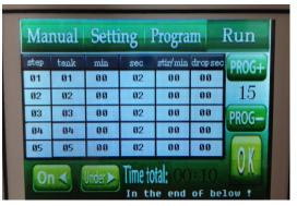
7) Press 'Run' key and press 'OK' key after checking. Screen should then appear as shown below.
