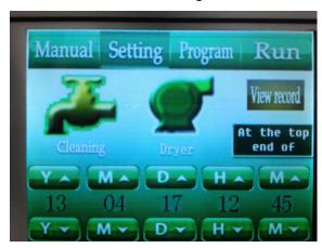
**5)** Press to switch between the options of ' end submerged (in the end of below) ' and ' end above station 2 (at the top end of)' to decide where the slide basket stays after staining is over according to user's need.
